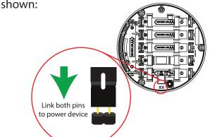
Combined sounder detectors are powered by changing the orientation of switch 1 as shown:
