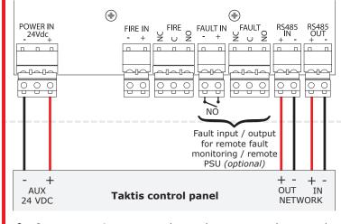
• Once connections are made, apply power to the control panel.
