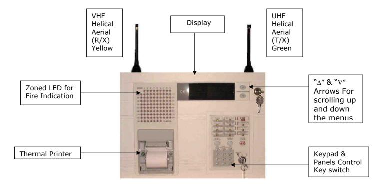
CONTROL PANELS ARE SUPPLIED WITH ALL DETECTOR ZONES IN TEST. PLEASE REFER TO SECTIONS 12 OR 14 IN THIS MANUAL TO MAKE ACTIVE.
