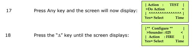
If you want to test another sounder repeat from step 13. If you have finished testing press the "NO" key until your back to the main screen (shown below). Then turn the key switch to the "OFF" position.
