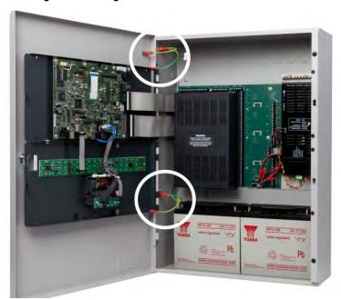
Remove the ribbon cables shown from the LCD Main Processor Board. The cables can be reconnected to the LCD Main Processor Board during the re-assembly process.
