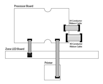
The fixed LCD Main Processor Board, optional Zone LED Board and optional Printer are mounted on the cabinet-lid of the FACP.
