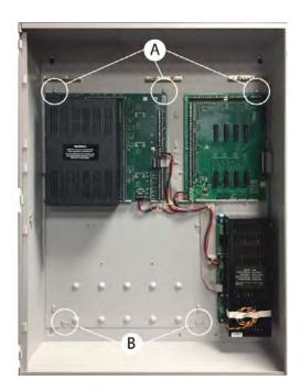
To remove the Chassis from the Cabinet-Box:
