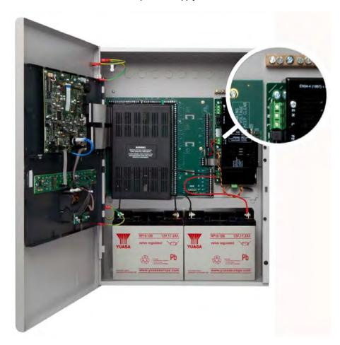
Dip Switches are located on the outer edge of the 5.25 Amp Power Supply. Dip switches of the 5.25 Amp Power Supply are located in a similar location as the 10.25 Amp Power Supply.
