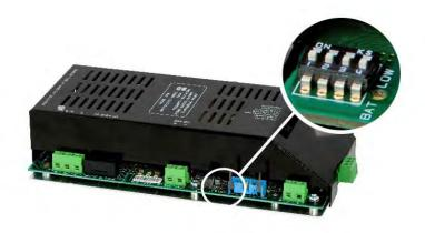
Figure 2-17 Dip Switch Position
