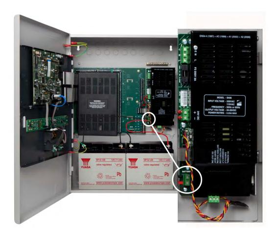
The series connection illustrated above provides the 24 volt standby voltage required by the Fire Control Panel. Do not connect the two batteries in parallel. A parallel connection will not provide the 24 volts required for operating the FACP in a standby condition.
