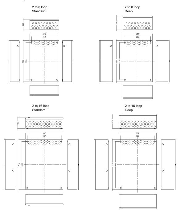
Drill four holes in the premises-wall according to appropriate dimensions identified above and then fix the empty cabinet to the wall using the mounting hardware to secure it.
