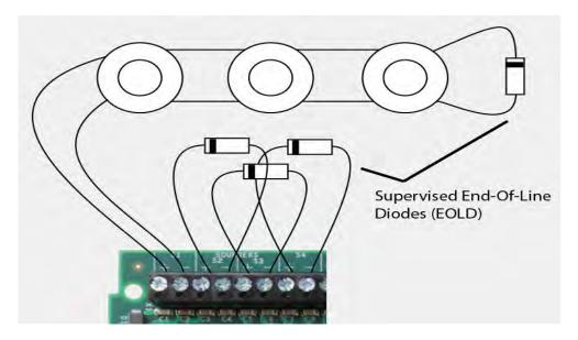
Synchronised device connections to the FACP require special conditions when installing audible and visual Sounders:
