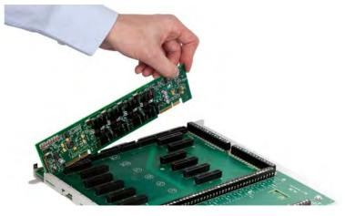
7 Rotate the circuit board until all conductors are securely inserted into connectors of the Chassis.
