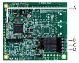
NOTE Do NOT wire to terminals B. C & D - use terminals on Back Board - See "Main Back Board" on page 5.
