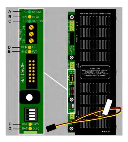
Status indicators of the 10.25 Amp Power Supply are identical to those of the 5.25 Amp Power Supply.
