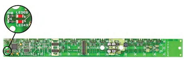
Zone indicators are not shown on the component-side image above. Zone indicators are located on the opposite side of the circuit board.
