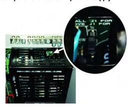
To provide 230 VAC operation, remove jumper-J1 from the circuit-board of the power supply.
