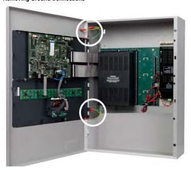
**6** Remove the two ribbon cables from the LCD Main Processor Board.
