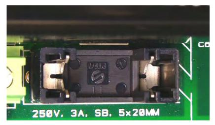
Replacement fuses must match the types originally fitted on the FACP.
