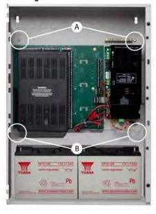
To remove the Chassis from the Cabinet-Box:
