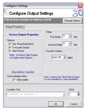
**NOTE:** If a loop sounder is controlled by a cause and effect operation, then the Tech Alarm tone will be used when the sounder is energised.
