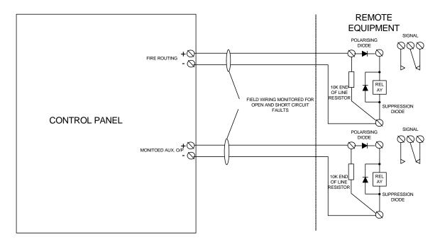
Connections to the remote equipment should be as shown above. It is important if the device at the receiving end is an electromagnetic device such as a relay that polarising and suppression diodes are fitted to prevent operation of the device in the normal condition and to suppress any interference generated by the device when it operates.
