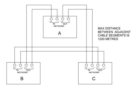
Network boards are fitted with isolators, which disconnect faulty sections of cable and allow the network to continue working by using the return path so it is most important that this wiring configuration be adhered to.
