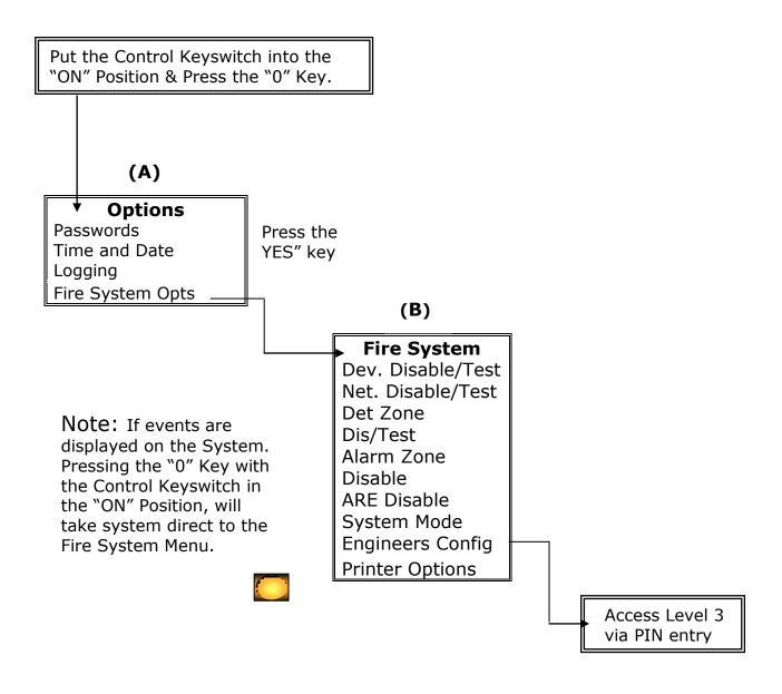
To scroll through the menus, use the " $\Delta$ " and " $\nabla$ " scroll buttons. To enter a menu position the required option between the > and < cursors on the screen and press the "YES" key.
