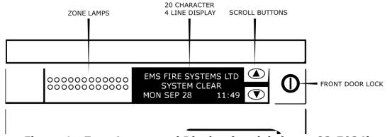
Figure 1 - Zone Lamps and Display (model shown 83-5024)
