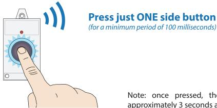
Note: once pressed, the device will continue to transmit for approximately 3 seconds after the button has been released.
