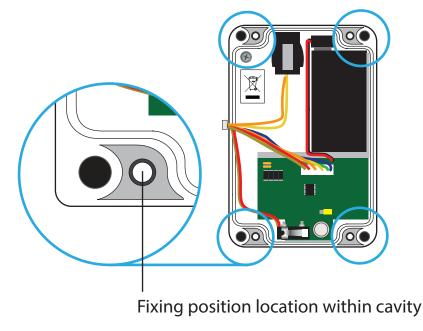
Note; if installing a device with air switch (7920/AS), an additional hole will need to be drilled to accommodate the device's air switch tube socket on the back of the box. See below.
