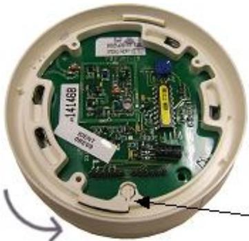
Press the plastic release button and turn anti-clockwise to as shown left to remove the base.
