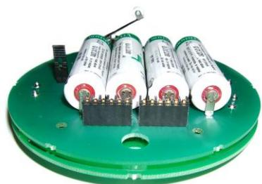
Once the base has been removed, take out the three battery board fixing screws, (as shown in figure 1).
