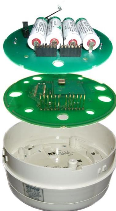
Now replace the battery board with a new one and reassemble the detector.
