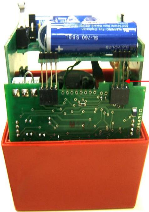
The battery board slots onto the other board using the connectors as shown. Firstly disconnect these.
