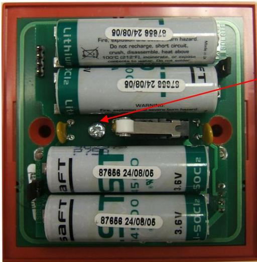
Remove this screw to release the callpoint battery board from the casing.
