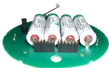
The battery board can now be separated from the transmitter / processor board. Remove carefully without damaging the pins.
