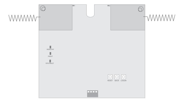
**Reset Button**; the reset button is used to reset the Radio Cluster Communicator.
